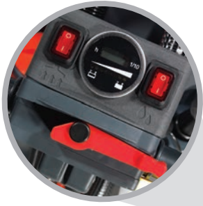
Control panel provides an hour meter and monitors the battery status
